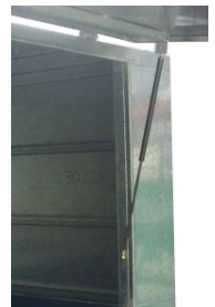
gas struts are standard inclusion on pantec tops
